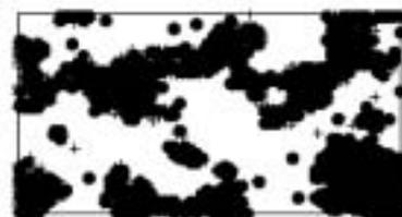
A 150x90 fragment of the lattice showing the patterns obtained in simulations of oscillations in the NO-CO reaction on Pt(100). The black and white regions correspond to the (1x1) and "hex" phase, respectively.
