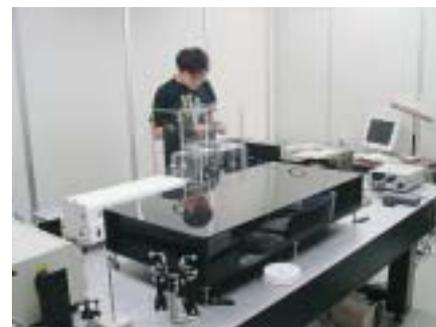
Fig. 2. Surface analysis with a broad band SFG system.
